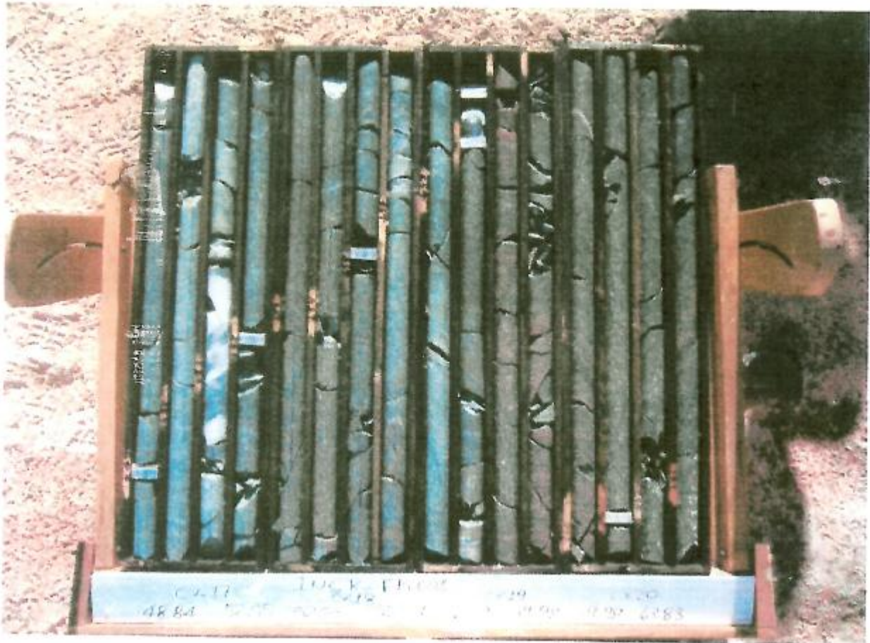
Image 19: Borehole DH01 - testimony NQ of the target Carrapato, Zé Padeiro
